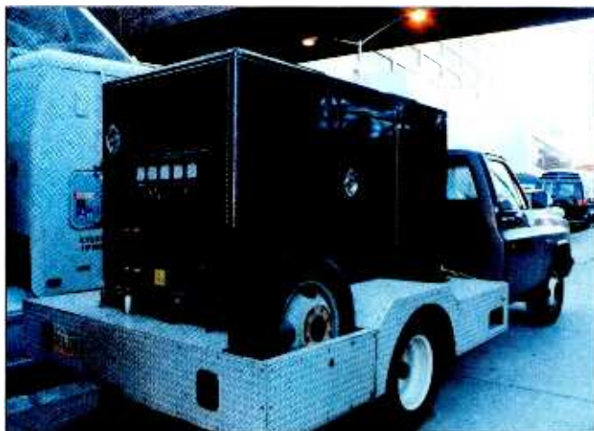
The capacity of this portable, diesel-powered generator is 166A, three-phase (500A total, single-phase). Its housing is felt-lined for quiet operation.
